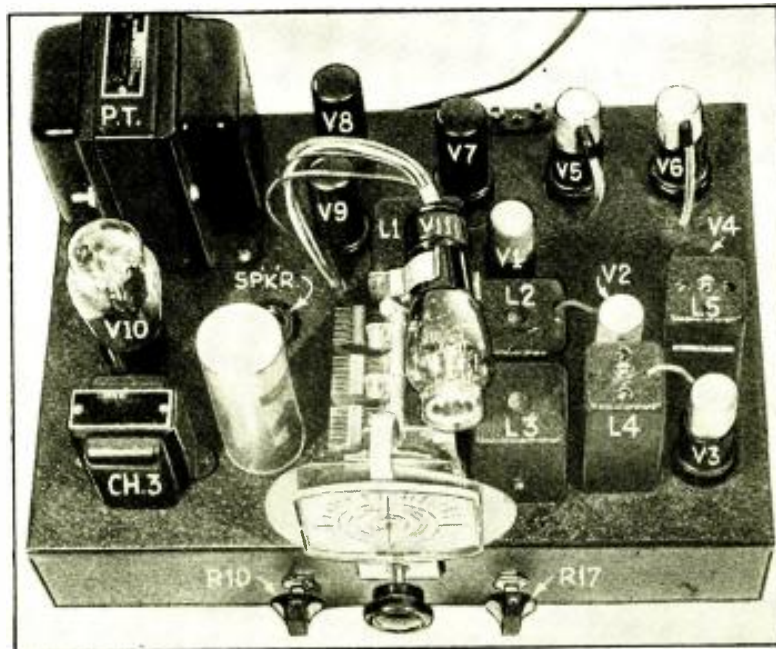
Fig. A. Chassis layout of the 11-tube broadcast set with "Syncrotronic" reproduction.
